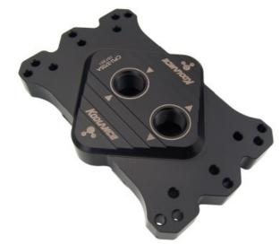
CPU-370SA is a lighter weight, lower priced version of Koolance's acclaimed CPU-370 water block. It includes a similar nickel-plated copper microfin cold plate (0.25mm fins, 0.30mm channels), o-ring sealed impingement plate, and a solid acetal top designed for AMD sockets.
