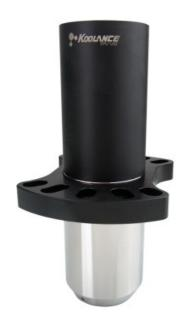
The Koolance CPU-LN2 is a "DIY" processor evaporator pot for liquid nitrogen or dry ice cooling. A nickel-plated solid copper cold plate is combined with a black acetal container. Mounting hardware includes a thick acetal top bracket, steel back plate, back plate insulating pads, and various mounting hardware. Moisture insulation is not included. The supplied bracket supports the following processor sockets:
