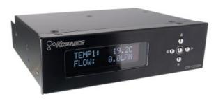
The CTR-CD1224 is a pump and fan speed controller and temperature monitoring unit in a 5.25in drive bay profile. The maximum pump output can be set for 12V or 24V. This unit incorporates a 2-line OLED display for user control and feedback.
