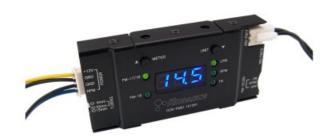
The DCB-FM01 displays flow rate or pulse signals from Koolance flow meters. Units can be toggled between liters per minute, gallons per minute, or raw impeller pulse rate (Hz). Pulse rate conversion can also be manually configured on the DCB-FM01 for custom flow meters (required for INS-FM14). An aluminum mounting bracket is included for computer 5.25in drive bay installation.
