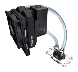
Koolance's DIY kit offers enthusiast-level thermal performance with an all-in-one form factor. ICM-PC30A includes the top-rated Koolance CPU-380A (AMD) water block, copper 30-FPI radiator and fan, PMP-300 pump, reservoir, and all necessary fittings and tubing. Simply select your desired coolant bottle (sold separately), and add some assembly. The kit's mounting bracket is adjustable, allowing a full size radiator and pump to fit most computer chassis with a rear 120mm fan location.
