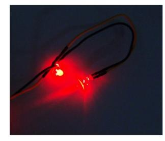
Koolance dual ultra bright LED's with a single 4-pin Molex connector. 3mm wide. Requires 12VDC input. Total length = 43.8cm (17.25") with 10.8cm (4.25") between LED's.
