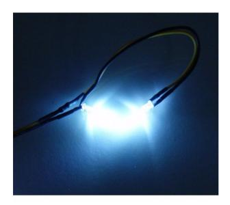
Koolance dual ultra bright LED's with a single 4-pin Molex connector. 3mm wide. Requires 12VDC input. Total length = 43.8cm (17.25") with 10.8cm (4.25") between LED's.
