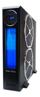
The ERM-2K3U continues Koolance's "ERM" series of dedicated liquid cooling systems for special thermal applications. It can provide up to approximately 2000W of potential heat dissipation, and is housed in a lightweight aluminum enclosure. A prominent white LED-lit reservoir displays the coolant level, combining a waterfall effect when placed upright.
