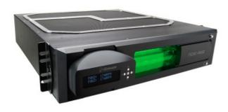
ERM-3K3UC is a rack-mountable or free standing ambient liquid cooling system. This model contains a large nine x 120mm fan copper/brass radiator, providing roughly 2600W of cooling with a 25°C ambient delta. Just add tubing, fittings, coolant, and connect to your cold plate(s).
