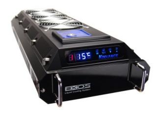
EX2-1055 is an ambient liquid cooling system designed with features for computer cooling. This model contains a triple x 120mm fan aluminum radiator, providing roughly 900W of cooling with a 25°C ambient delta. Just add tubing, fittings, coolant, and connect to your cold plate(s).
