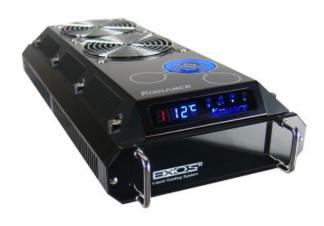
EX2-755 is an ambient liquid cooling system designed with features for computer cooling. This model contains a dual x 120mm fan aluminum radiator, providing roughly 590W of cooling with a 25 °C ambient delta. Just add tubing, fittings, coolant, and connect to your cold plate(s).
