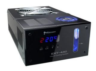
EXT-440CU is a compact ambient liquid cooling system designed with features for computer cooling. This model contains a single x 120mm fan copper/brass radiator, providing roughly 400W of cooling with a 25 °C ambient delta. Just add tubing, fittings, coolant, and connect to your cold plate(s).
