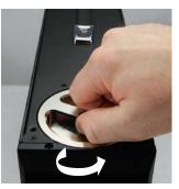
To avoid spilling, a large funnel is recommended. Coolant should be filled to about 1/2-inch (13mm) from the top of the reservoir. **Never completely fill or "top-off" the reservoir.** An air gap is needed to accommodate thermal expansion of the liquid.
