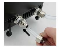
Squeeze the tube while pushing it firmly over the fitting. The tubing should completely cover the fitting. This step can be made easier by first dipping the end of the tubing in warm water.
