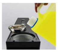
Slowly fill the system with coolant. **To maintain the product warranty, use only Koolance approved coolant.** Many alternative liquids and additives can cause permanent damage to the system through chemical reaction, corrosion, biological growth, high thermal expansion, viscosity, etc.
