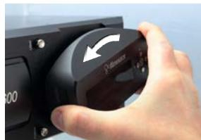
The display panel can be adjusted for these orientations by gently pulling it forward while rotating.
