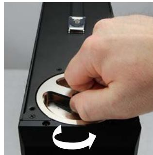
To avoid spilling, a large funnel is recommended. Coolant should be filled to about 1/2-inch (13mm) from the top of the reservoir. **Never completely fill or "top-off" the reservoir.** An air gap is needed to accommodate thermal expansion of the liquid.
