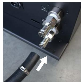
Squeeze the hose while pushing it firmly over the fitting. The hose should completely cover the fitting. This step can often be made easier by first soaking the end of the hose in warm water for a few minutes.
