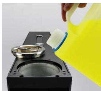
This cooling system requires approximately **3 liters (0.8 gallons)** of coolant, plus additional coolant for externally attached components and hose.
