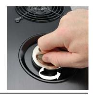
To avoid spilling, a large funnel is recommended. Coolant should only be added up to the line labeled "Max Fill". **Never completely fill or "top-off" the reservoir.** An air gap is needed to accommodate thermal expansion of the liquid.
