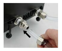
Squeeze the tube while pushing it firmly over the fitting. The tubing should completely cover the fitting. This step can be made easier by first dipping the end of the tubing in warm water.
