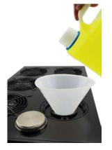
Slowly fill the system with coolant. To maintain the product warranty, use only Koolance approved coolant. Many alternative liquids and additives can cause permanent damage to the system through chemical reaction, corrosion, biological growth, high thermal expansion, viscosity, etc.
