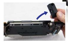
Place the o-rings included with your bridge blocks into each of the grooves beneath it. This must be done for both bridge blocks.
