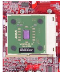
Socket alignment for left AMD processors
