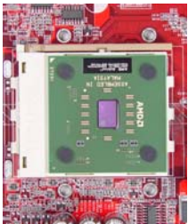
Socket alignment for right AMD processors
