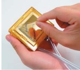
Insert the temperature sensor into *either* bottom groove on the CPU cooler. The sensor is required for proper fan speed control and system safety features.
