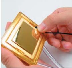
DO NOT attempt to install the temperature probe *in between* the processor and cooler. Despite its thin size, it will interfere with CPU contact or burn-out the sensor.
