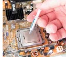
Apply thermal paste to the CPU directly.
