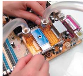
The temperature sensor should already be installed into the CPU Cooler.
