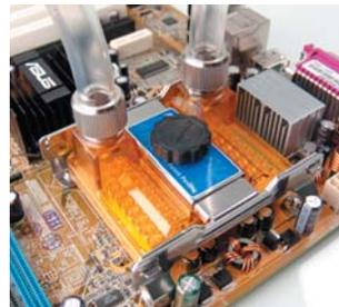
Check that the bracket clips are aligned in all 4 rail holes before installing the tension screw.
