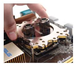
Use either 2 or 4 springs and thumb nuts (depending on socket type) to secure the cooler against the processor.
