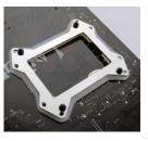
Above the motherboard, place a plastic washer around each mounting post. Hand-tighten a metal nut onto each post above the washer to hold
