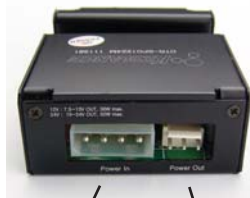
Power In (12VDC) Power Out (Pump, Fan, etc.)
