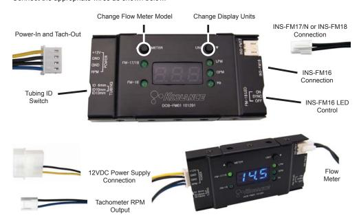
With the included wiring harness, connect a 12V DC power supply input. Optionally, plug the tachometer output wire to a header capable of reading fan RPM values. RPM values from the DCB-FM01 will correspond with milliliters per minute.
