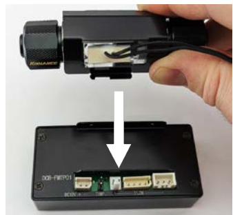
Hook the lower bracket tab into the display
