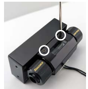
Secure with two screws on top
