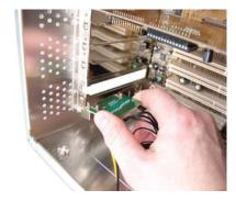
Install the Slot Adapter into any available rear card slot in your computer.
