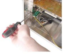
From the rear of the case, carefully feed both ends of the liquid tubing through the Slot Adapter and into the chassis.
