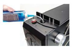
Slowly fill the system. To maintain the product warranty, use only Koolance approved coolant. Many alternative liquids and additives can cause permanent damage to the cooling unit (through
