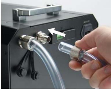
Tighten the connection by sliding the compression nut down over the fitting and screwing securely. For hose barbs, use pliers to move it into the proper position before releasing.
