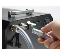
Squeeze the tube while pushing it firmly over the fitting. Tubing should completely cover the fitting or barb.
