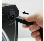
Power on the cooling unit, and increase the pump speed to move coolant if needed. When most of the air has been pushed out of the tubing, the liquid noise will decrease. This process can take several minutes, depending on the filling technique and components attached to the cooling system.
