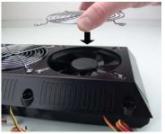
Place all 3 fans onto the mounting posts with labels facing down (airflow moving down into the radiator).
