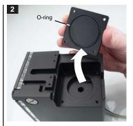
Place the pump in the desired location and attach with the longer screws included with the RP-402X2. The pump wire must exit the back end of the reservoir.
