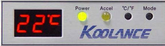
Mode 1 operates your system at 45% power until the temperature reaches 45°C (113°F), then increases to 100% power.
