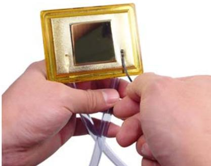
Insert the temperature sensor into *either* bottom groove on the CPU cooler.
