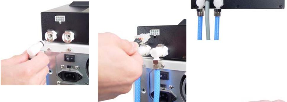
If you are having difficulties inserting quick-release nozzles into the rear connections, press the top valve button to close the valve. The nozzle will not fit into the Exos if the valve is open.
