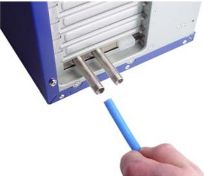
From the rear of the case, carefully feed both ends of the liquid tubing through the tension springs and into the chassis.
