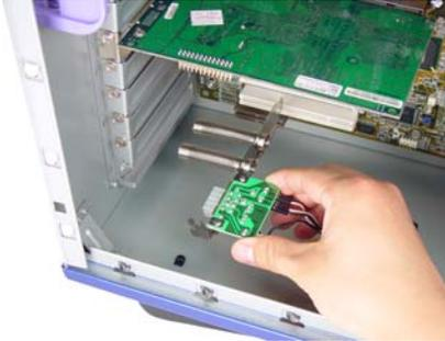
Install the Interface Adapter from the inside of the case, guiding the tension springs out the back of the slot. The Interface Adapter may be installed into any available rear card slot in your computer.
