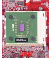
Socket alignment for left AMD processors
