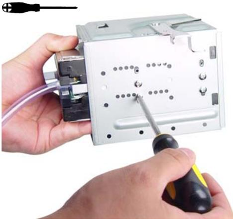
The second drive is mounted upside-down to the cooler, held in place via its own side-mounting screws.
