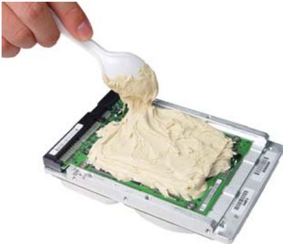
Using the mixing utensil, apply the encapsulate to the largest heat-producing components: the spindle motor and primary circuit chips on the bottom side of the drive.
