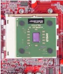
Socket alignment for right AMD processors
