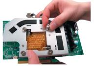
Finally, screw-tighten a mounting nut firmly to each metal post.
