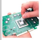
Additional thermal paste will likely be required on the GPU chipset and RAM modules after removing the original heat sinks.
