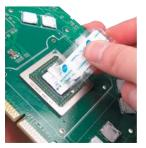
Remove all hardware nuts, washers, and metal posts from the Koolance black rear brace. Then, insert it into the back side of the video card.
