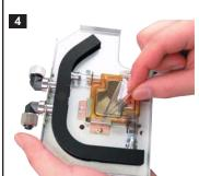
Remove the protective film from the bottom of the chipset cooler and mount it to the video card.
