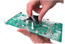
On front of the card, place plastic insulating washers on each of the 4 brace mounting screws.
