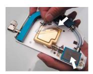
Remove the protective film from the bottom of both chipset coolers, and the PCI-Express controller chip (on the main cooler only).
