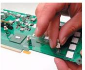
insulating washer over the mounting screw.
