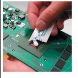
Thermal paste will be required on both GPU chipsets, all 16 RAM modules, and the PCI-Express controller chip (on the main board) after removing both original heat sinks.
