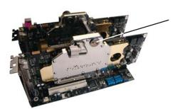
Two G1/4 "caps" are included with the VID coolers which can be placed opposite the desired nozzle locations.
