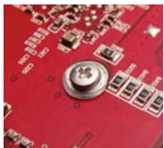
Koolance-Supplied Screw and Insulating Washer
