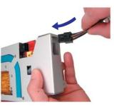
Fold the enclosure closed. The long screws should fit through both holes in the VID-AT1-V06 back plate.
