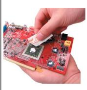
Spread the thermal compound evenly to cover each chip using the paste packet, or a piece of thick paper (such as a business card).
