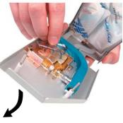
Place the video card into the cooling enclosure. There are 2 long screws on the enclosure which must be inserted through the card.
