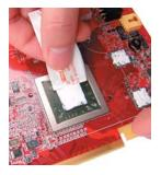
Open the VID-AT1-V06 enclosure and remove the protective film from the bottom of the chipset cooler.
