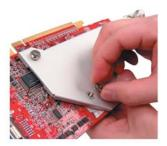
When installing your Radeon card, the power supply connection can be inserted through the back of the VID-AT1-V06.
