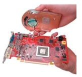
Apply fresh thermal paste to the main chipset, taking care *only to coat the raised center core*. The outer portion of the chipset and metal frame do not require thermal compound.
