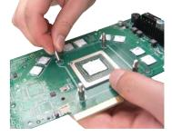
NOTE: Video card RAM chips are not perfectly flat with one another. To make sure your VID-NV1-L06 is making the best contact possible for your card, remove the cooler and examine the distribution of thermal paste.
