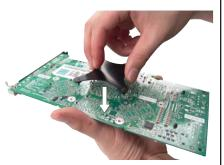
On front of the card, place plastic insulating washers on each of the 4 brace mounting screws.
