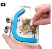
Remove the protective film from the bottom of the chipset cooler and mount it to the video card.
