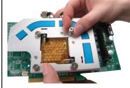
Finally, screw-tighten a mounting nut firmly to each metal post.
