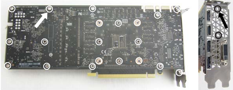
GTX 1080 Disassembly Screws (Bottom and Rear L-Bracket)
