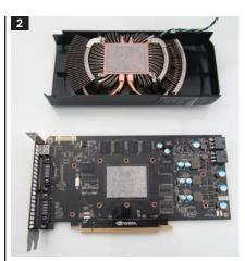
Carefully remove the heat sink. Original thermal paste may present resistance during removal.
