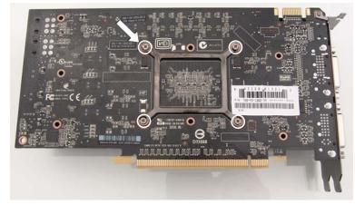
GTX 460 Disassembly Screws
