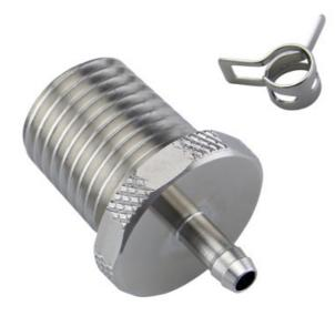
Single hose barb fitting for 1/8in (3mm) ID tubing. 1/4 NPT (tapered) thread. Includes hose clamp for 5mm (3/16in) OD tubing.
