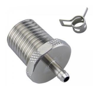
Single hose barb fitting for 1/8in (3mm) ID tubing. 1/4 NPT (tapered) thread. Includes hose clamp for 5mm (3/16in) OD tubing.
