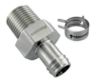
Single hose barb fitting for 3/8in (10mm) ID tubing. 3/8 NPT (tapered) thread. Hose clamp for 1/2in (13mm) OD included.
