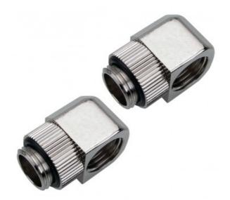
Create a swiveling 90 degree elbow bend using any Koolance G 1/4 BSPP (parallel) thread fitting. For a basic elbow fitting, the Koolance Coupling Adapter could also be used. Or for maximum adjustment, consider placing two swiveling elbow fittings together. Nickle-plated brass body, nickel-plated steel plugs. Fittings not included.
