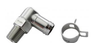
Single rotational angled fitting for 1/2in (13mm) ID tubing. 1/4 NPT (tapered) thread. Tube clamp for 5/8in (16mm) OD included.
