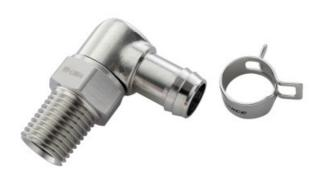
Single rotational angled fitting for 3/8in (10mm) ID tubing. 1/4 NPT (tapered) thread. Tube clamp for 1/2in (13mm) OD included.
