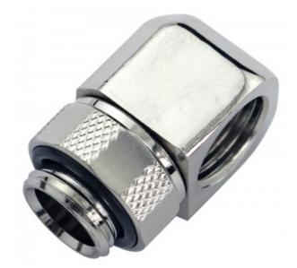
Create a swiveling 90 degree elbow bend using any Koolance G 1/4 BSPP (parallel) thread fitting. For a basic elbow fitting, the Koolance Coupling Adapter could also be used. Or for maximum adjustment, consider placing two swiveling elbow fittings together. Tube fitting not included.
