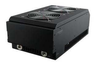
HXM-ALX1450 is a dual fan heat exchanger for Koolance's <u>ALX modular cooling systems</u>. When combined with an <u>RPM reservoir and pump module</u> (sold separately), the heat dissipation is approximately 1450W. Front fitting threads are G 1/4 BSPP, and the rear are 1/4 NPT.
