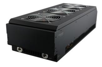
HXM-ALX2000 is a triple fan heat exchanger for Koolance's <u>ALX modular cooling systems</u>. When combined with an <u>RPM</u> reservoir and pump module (sold separately), the heat dissipation is approximately 2000W. Front fitting threads are G 1/4 BSPP, and the rear are 1/4 NPT.
