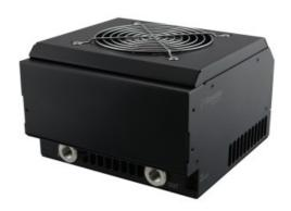
HXM-ALX750 is a single fan heat exchanger for Koolance's <u>ALX modular cooling systems</u>. When combined with an <u>RPM reservoir and pump module</u> (sold separately), the heat dissipation is approximately 750W. Front fitting threads are G 1/4 BSPP, and the rear are 1/4 NPT.
