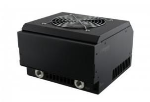
HXM-ALX750 is a single fan heat exchanger for Koolance's <u>ALX modular cooling systems</u>. When combined with an <u>RPM reservoir and pump module</u> (sold separately), the heat dissipation is approximately 750W. Front fitting threads are G 1/4 BSPP, and the rear are 1/4 NPT.
