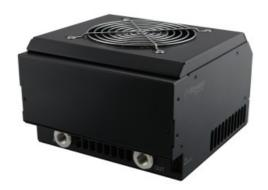
HXM-ALX750 is a single fan heat exchanger for Koolance's <u>ALX modular cooling systems</u>. When combined with an <u>RPM reservoir and pump module</u> (sold separately), the heat dissipation is approximately 750W. Front fitting threads are G 1/4 BSPP, and the rear are 1/4 NPT.
