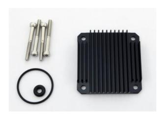
HTS-PMP401 is an optional aluminum heat sink for extra cooling of the Koolance PMP-400 pump and COV-RP400 fitting and reservoir base (both are required). It can assist in improving component reliability under high ambient temperature conditions.
