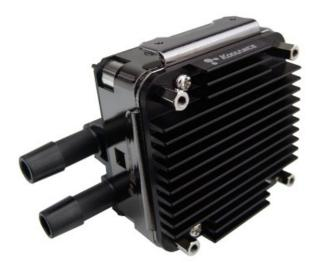
HTS-PMP400 is an optional aluminum heat sink for extra cooling of the Koolance <u>PMP-400</u> pump. This can assist in improving component reliability under high ambient temperature conditions. When assembled, the heat sink is in direct contact with the pump electronics via a thermal pad.
