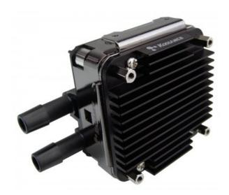
HTS-PMP400 is an optional aluminum heat sink for extra cooling of the Koolance <u>PMP-400</u> pump. This can assist in improving component reliability under high ambient temperature conditions. When assembled, the heat sink is in direct contact with the pump electronics via a thermal pad.
